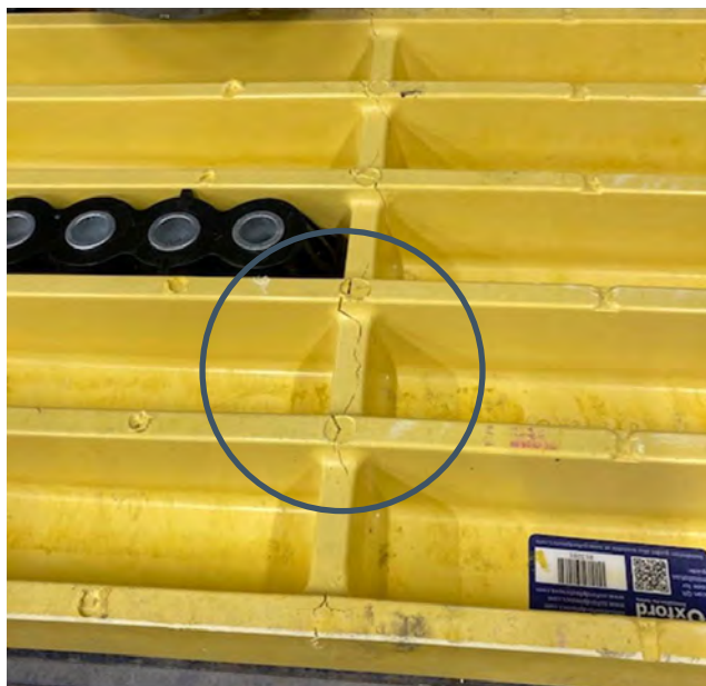
Crack along rib
